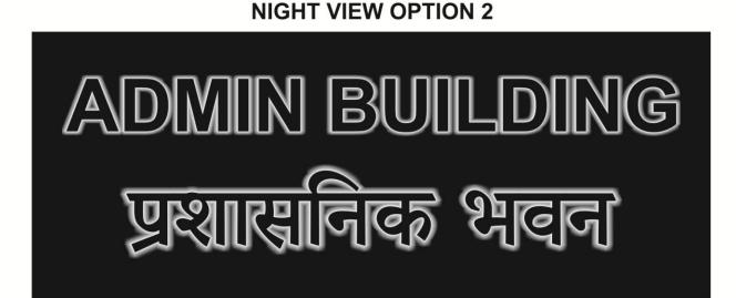
22 gaudge 1.5" raising S.S. Letters, 3mm Acrylic Chanel Letters on back of the letters to cover LEDs, White LED with 2 yrs. warranty, water proof power supply with 1 yr. warranty, fixing with Aluminium Clips & necessary electrical fittings
