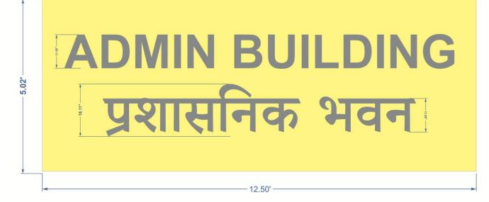
22 gaudge 1.5" raising S.S. Letters, 3mm Acrylic Chanel Letters on back of the letters to cover LEDs, Blue LED with 2 yrs. warranty, water proof power supply with 1 yr. warranty, fixing with Aluminium Clips & necessary electrical fittings
